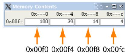
Figure 4: Memory display window for SEQ simulator
